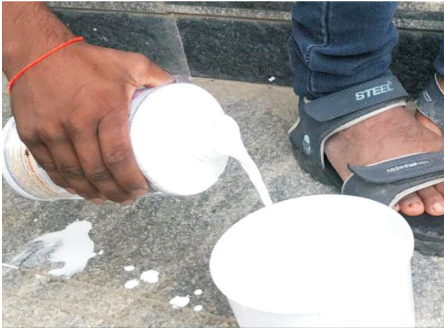
Figure 1. Chemical used for Membrane Curing
