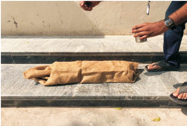
Figure 4. Sprinkling of Water on Prism Covered with Gunny Bag
